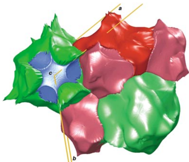
Figure 4. Atomic surfaces defined by the zero flux condition of the different atoms in the \text{Zn}_4\text{Sb}_3 structure viewed nearly along the c axis. The light shiny green basins along the c axis correspond to the “dimer” Sb atom. At the top of the Sb dimer a non-nuclear maxima (blue) fits exactly into the void. The red basin is the main Zn atom, the purple basins are the interstitial Zn atoms and the matt green basin is the \text{Sb}^{3-} ion.
